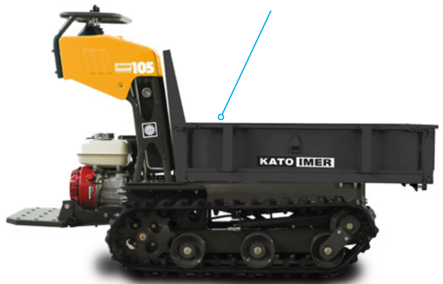
Loading bed with closed sides dim. LxPxH 900 x 620 x 200 mm
