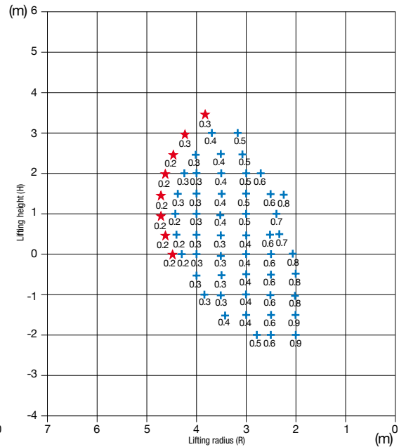
Side lifting, spanner contracted, with standard arm
