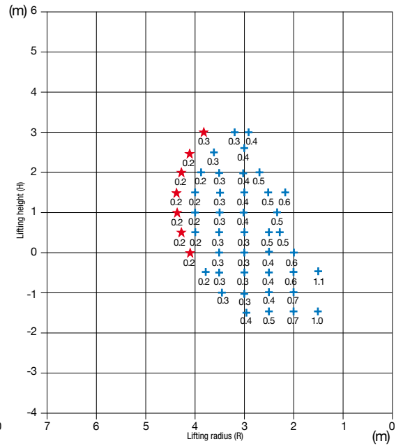
Side lifting with standard arm
