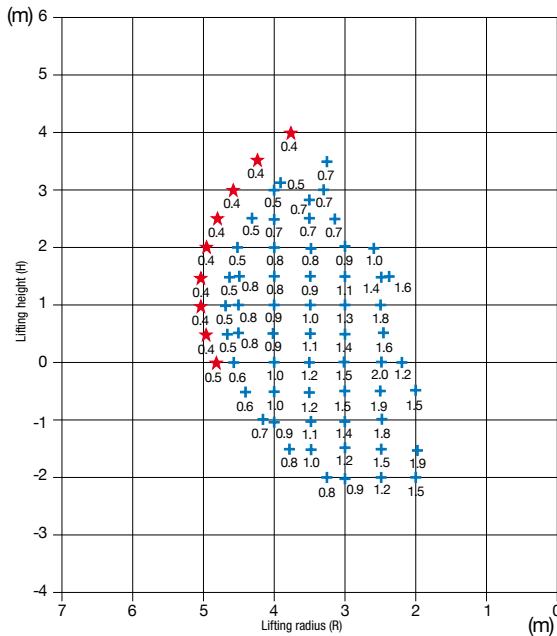
Front lifting, with blade on the ground, with standard arm
